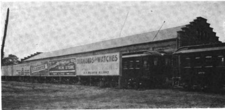
STORING CARS OUTDOORS. PROTECTING FENCE TO SHIELD THEM, PAID FOR BY ADVERTISING, STARK ELECTRIC
